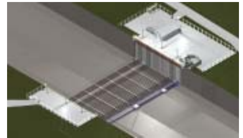
Early diagram of the electric Aquatic Nuisance Species barrier in Chicago.
