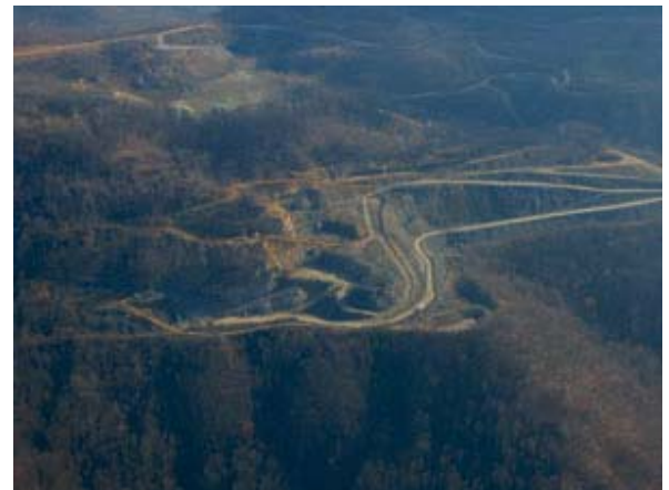
Zeb Mountain, TN “cross section” mining where waste rock is salvaged and used to restore the mountain’s contour (Greenwire Photo by Daniel Cusick).
