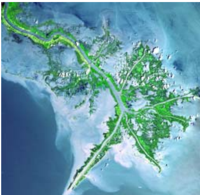
Satellite view of the Mississippi River Delta showing how barge canals and flood control projects have isolated the river from its floodplain wetlands and distributaries. (NASA Photo)
