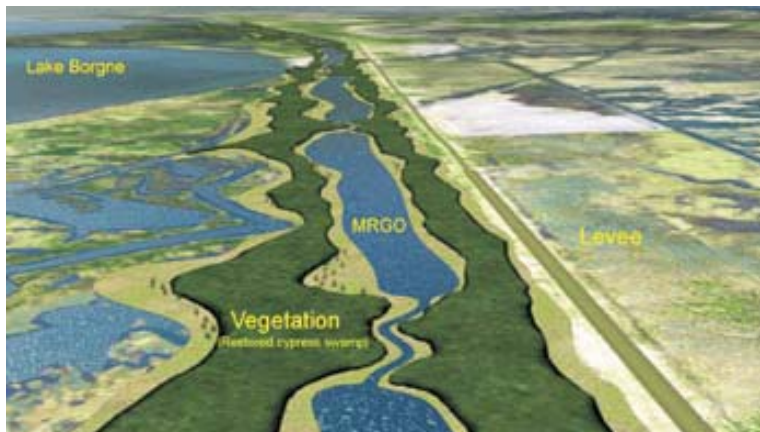
Diagram showing how the MRGO would look if its banks and the cypress swamps near its levees were restored. Environmental Defense image.
