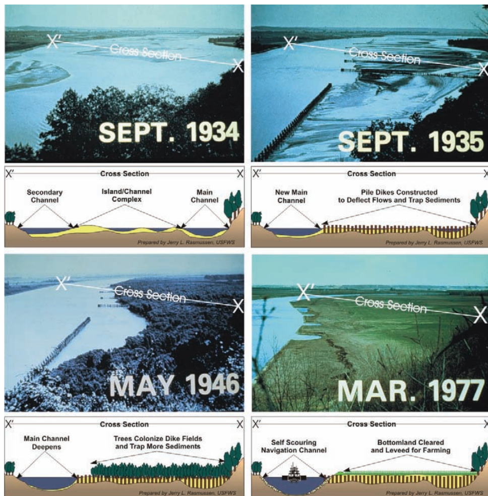
Channelization of the Missouri River at Indian Cave Bend near Rulo, NE between 1934 and 1977 with graphic cross sections depicting the process in action. USACE photos.
