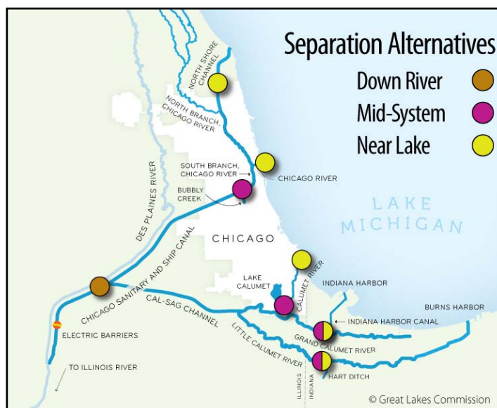
Suggested alternative barriers for separation of the Great Lakes from the Mississippi River Basin - Great Lakes Commission graphic
