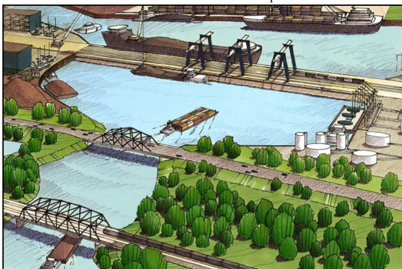
Diagram showing how a hydrologic separation along the Calumet River (top) could still allow for transfer of cargo and shipping along the CAWS (bottom). Sketch taken from the GLC Study Report . (HDR, Inc. sketch).
