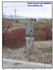
Example of a ground based cloud nucleating generator. A propane flame is used to vaporize the seeding solution, which is composed of silver iodide mixed in acetone. The vaporized silver iodide then re-crystallizes in the cold air, forming millions of tiny particles which are intended to serve as ice nuclei. The generators are positioned to maximize the number of silver iodide crystals that reach the critical regions of passing storms. North American Weather Consultants, Inc. Photo.
