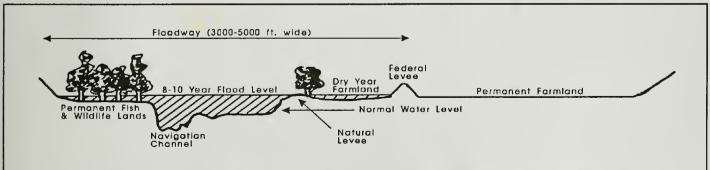
Proposed floodway works with nature storing flood water in floodplains, meeting multiple use objectives, while protecting prime developed lands, urban, and industrial areas from high river stages.
