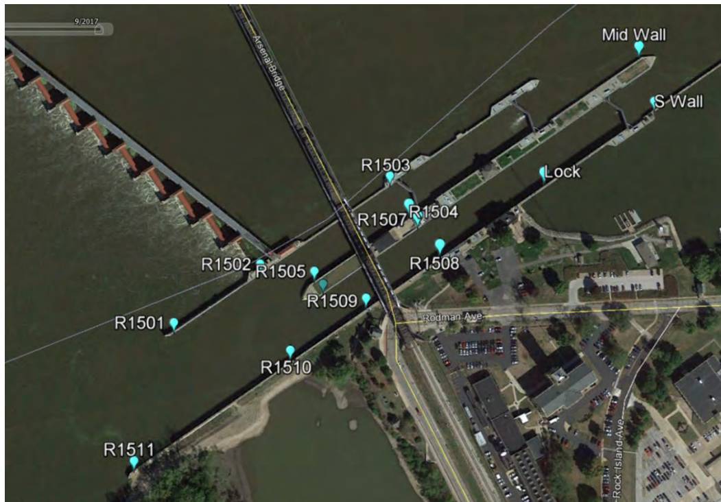
Location of receivers completing the Vemco array in the lock approach at Lock 15.
