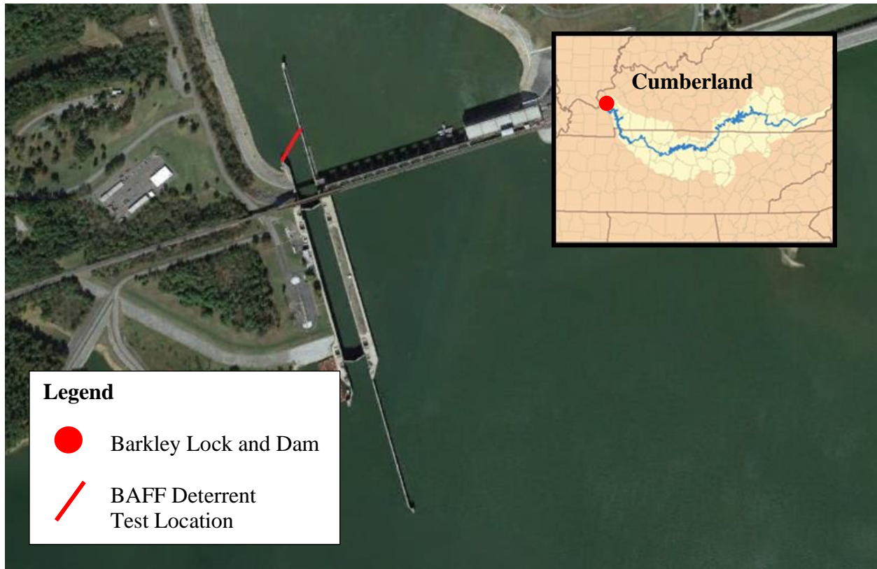
Figure 1. Location of Bio-Acoustic Fish Fence (BAFF) deterrent system being tested at Lake Barkley Lock and Dam on the Cumberland River.
