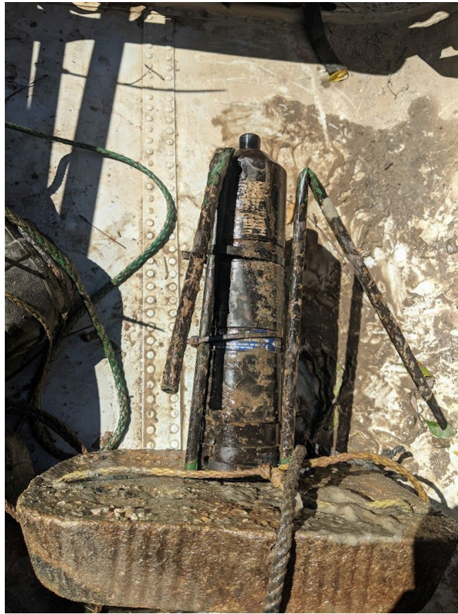
Figure 3. A VR2Tx acoustic receiver attached to the concrete anchor and float lines and used to passively record movements of acoustically tagged Silver Carp Hypophthalmichthys molitrix that pass the receiver.
